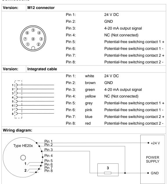
Fig. 7: Wiring diagram
