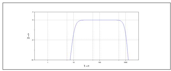
Fig. 2: Typical frequency response 10 Hz–1000 Hz
