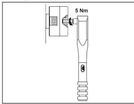
Tighten housing cover with torque wrench (2)
