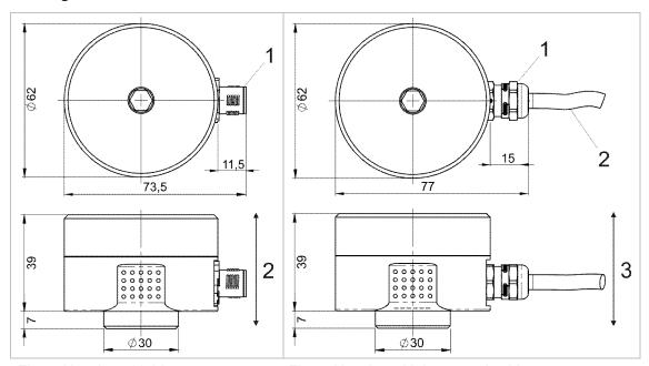
Fig. 4: Housing with M12 connector
