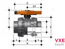
**VXEAC** Easyfit 2-way ball valve with female ends for solvent welding, ASTM series
