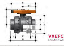
Easyfit 2-way ball valve with BSP threaded female ends
