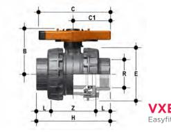
**VXENC** Easyfit 2-way ball valve with female ends, NPT thread
